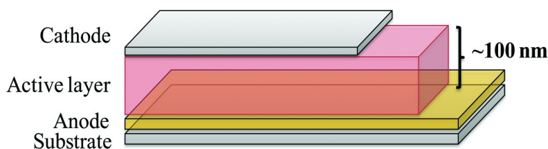
Figure 1. Representative configuration of an OPV device. The active layer is comprised of a blend of electron-donor and electron-acceptor organic semiconductors.
